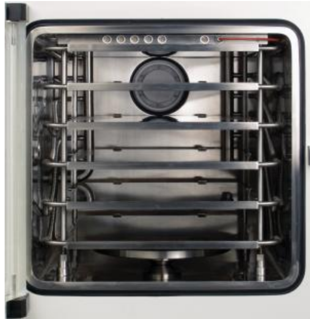
Drying chamber: 120 mm diameter valve to ice condenser
